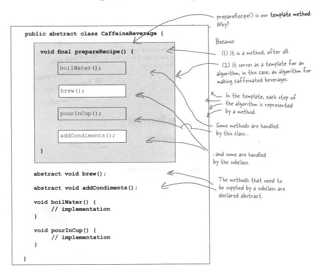
The Template Method defines the steps of an algorithm and allows subclasses to provide the implementation for one or more steps.
