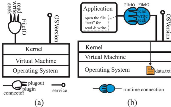
**Figure 1.** (a) Building blocks of the  $\mu$ KVM (b) Runtime connection on connectors
