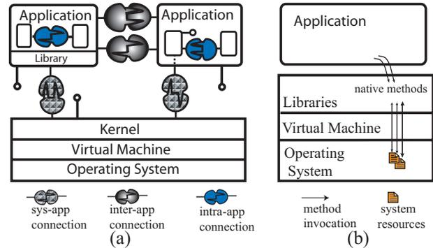
**Figure 2.** (a) The  $\mu$ KVM runtime overview and (b) J2SDK Runtime
