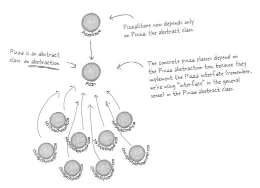
After applying the Factory Method, you'll notice that our high-level component, the PizzaStore, and our low-level components, the pizzas, both depend on Pizza, the abstraction. Factory Method is not the only technique for adhering to the Dependency Inversion Principle, but it is one of the more powerful ones.
